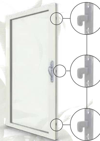
Every Restorations Sliding Door incorporates a concealed three-point locking system, which is recessed in the door panel. Three locks simultaneously engage into the keepers in the door jamb when the door is closed.
